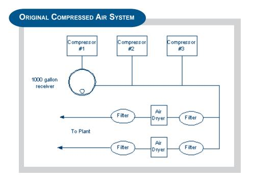
system's dynamics—the interaction of airflow rate with the inherent resistance of the pipeline and air system components. Because of the increased resistance caused at times by the filtration components, the compressed air system experienced a pressure drop of 10 to 15 psig. This was one of the main reasons why the compressor discharge pressures had to be kept at 95 to 105 psig.
